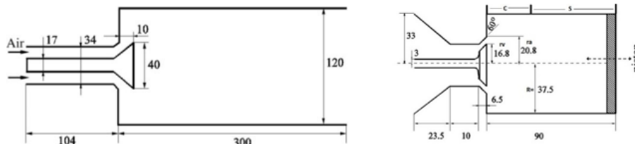
Fig. 3. Validation model 1 and 2 geometrical details (dimensions in mm) [26, 28]
