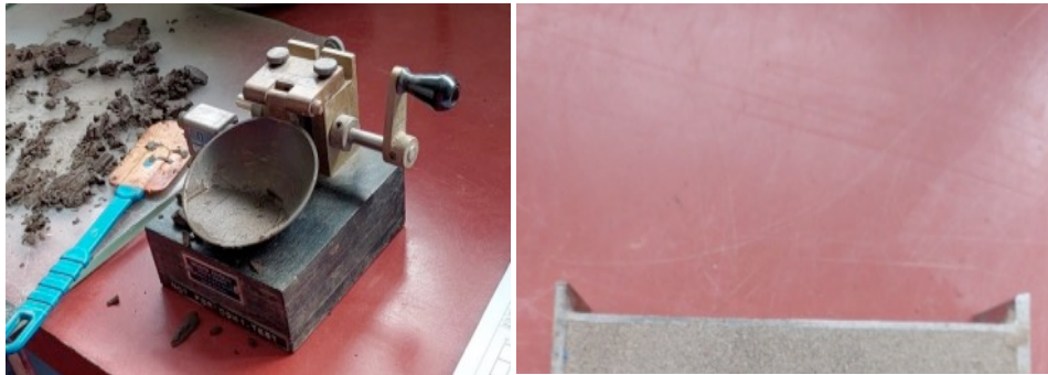
Fig. 4. (a) Casagrande cup containing soil for the liquid limit test (b) shrinkage mold containing soil for shrinkage limit test.
