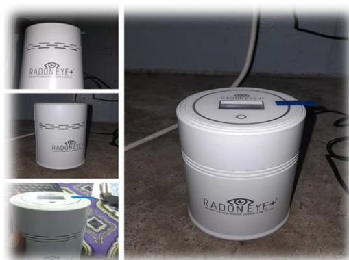
Fig. 1: Radon Eyeplus2 instrument for the measurement of Radon gas
